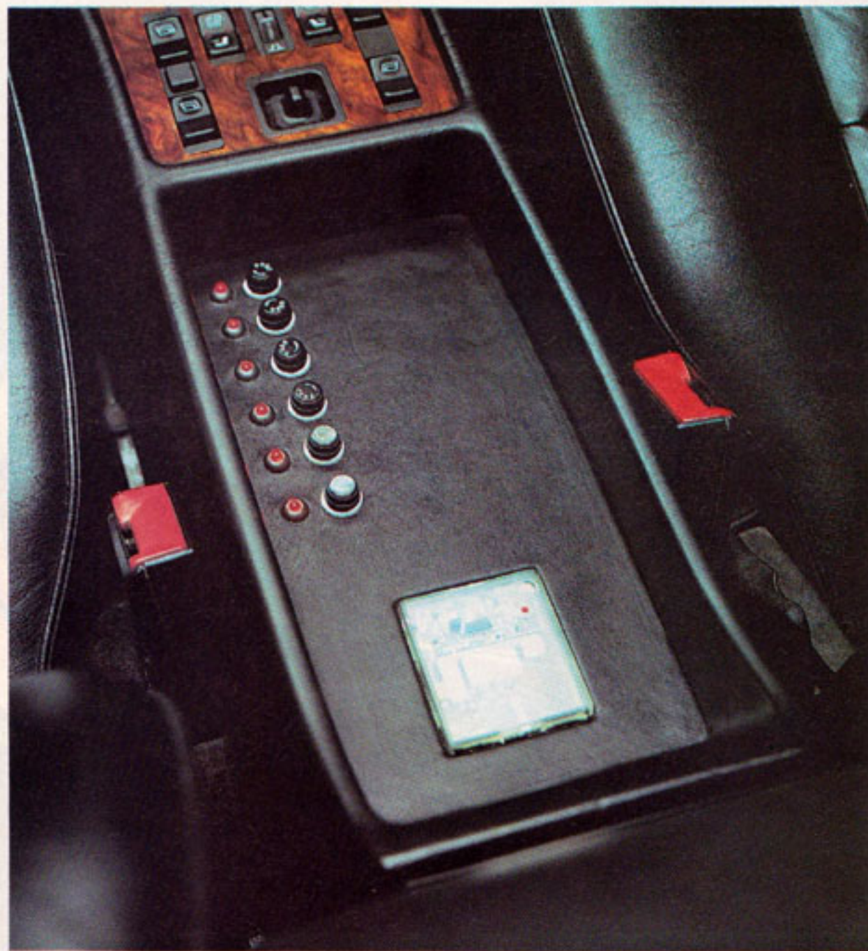
A chorus line of LEDs and fuses and a proximity sensor reside within the leather-clad armrest.
